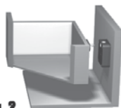
Fig. 2 Back of Drawer Installs using Locking Pin with Alarm function. Requires external reader
